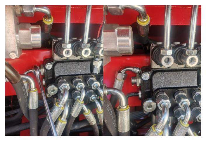
3. Unscrew the hexagon nipple as shown in the picture and insert it where the plug was removed.
