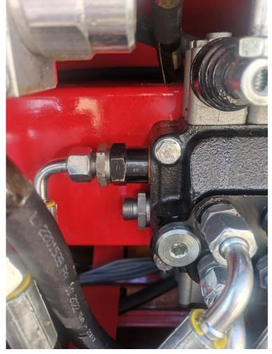
7. Loosen the T-nipple as shown in the picture and put an extra T-nipple between the one that was loosened and the valve.
