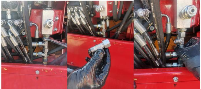
8. Install a new hose between the new hexagon nipple and the T-nipple.
